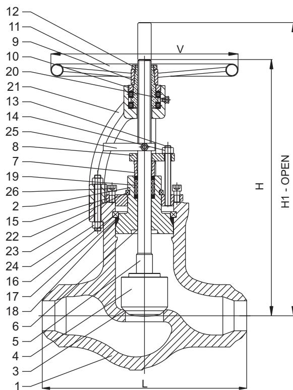
If higher, valve to be mounted with gear operator or with pressure above the disc and fitted with external or internal bypass.
